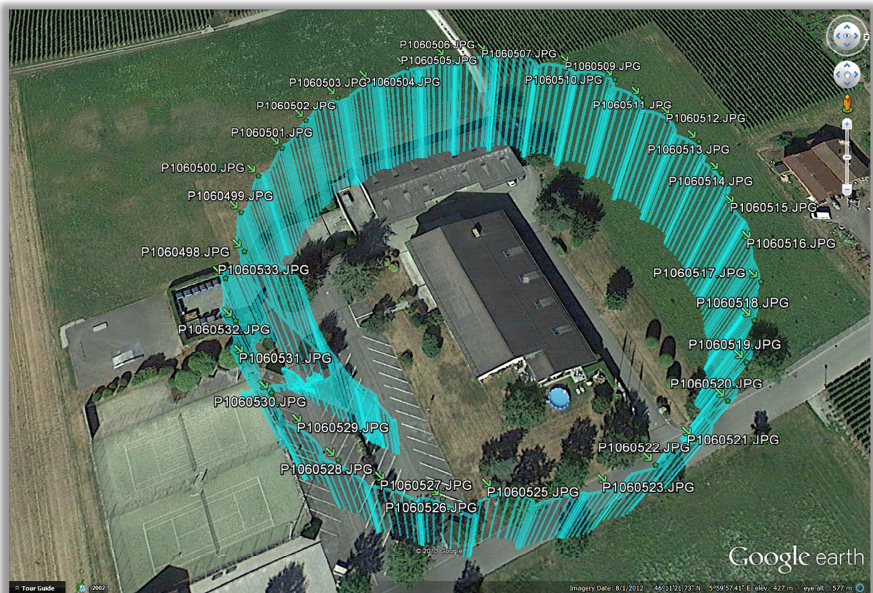
Figure 4: AscTec Falcon 8 log of flight to model the building / area of interest.
