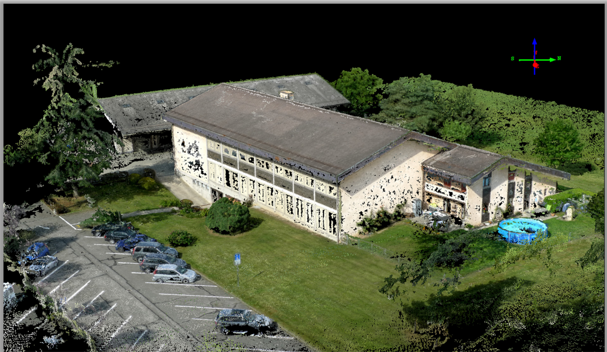
Figure 6: AscTec Falcon 8 & Pix4D resulting point cloud.
