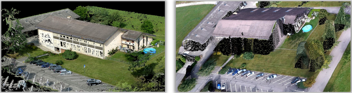
Figure 27: Typical point clouds produced by copter (left) and fixed wing (right) platforms.
