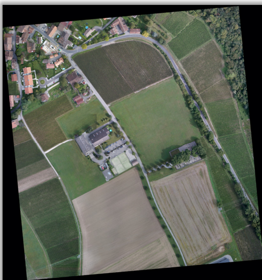
Figure 10: Gatewing/Trimble UX5 resulting ortho-rectified maps (regular and close infrared camera system).
