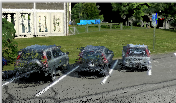
Figure 7: AscTec Falcon 8 & Pix4D details of resulting point cloud.
