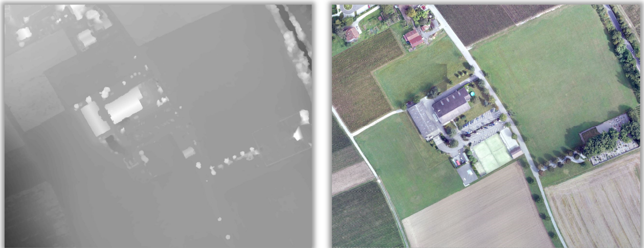
Figure 28: Typical Digital Surface Model (DSM) and ortho-rectified map (details) generated by fixed wing platforms.
