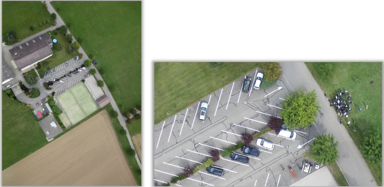
Figure 20: senseFly eBee nadir picture (left) and detail of resulting ortho-rectified map (right).
